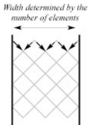
Figure 5: Diagram showing the boundaries for a 6-element braid.
